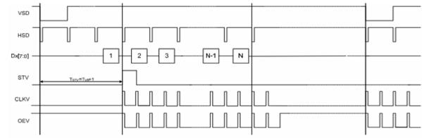
Vertical Timing Diagram DE (Dual Gate)
