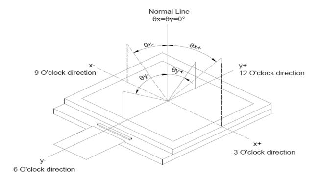
Note (2) Definition of Contrast Ratio(CR): measured at the center point of panel
