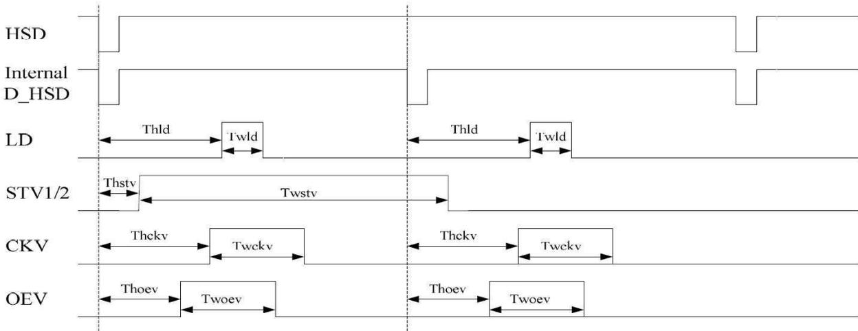
**AC Electrical Characteristics** (VDD =3.0~3.6V, VDDA=6.5~13.5V, AGND=DGND=0V, TA= -20~85 $\geq$ )
