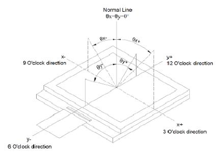
Note (2) Definition of Contrast Ratio(CR): measured at the center point of panel
